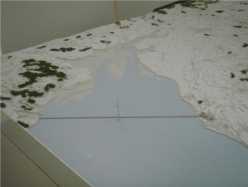
Fig. 1. Section of model showing 'tidal gateway' across Solway Firth.
