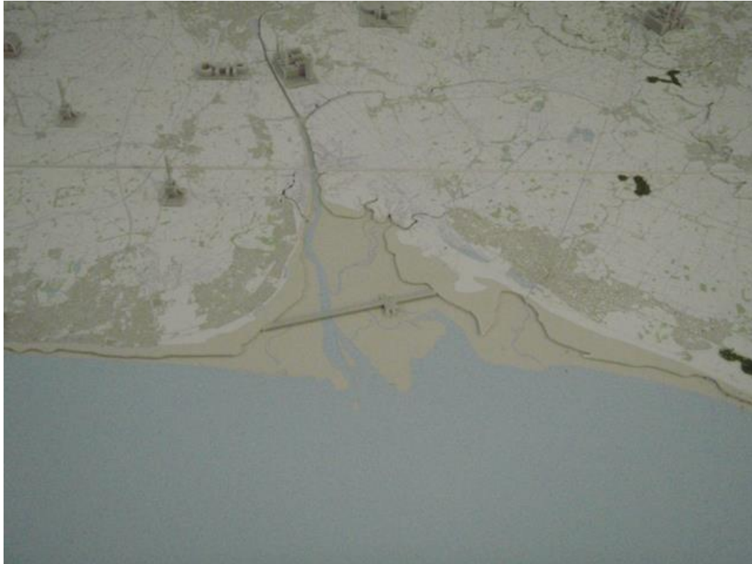
Fig. 3. Section of model showing 'tidal gateway' across Ribble Estuary.
