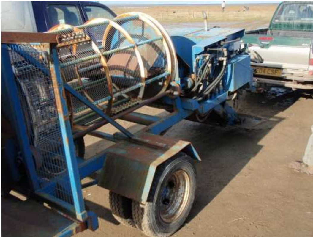
Figure 3. Towed “dry” cockle dredge showing wire drum riddle.
