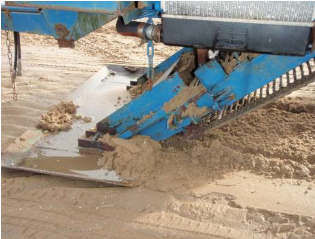
Figure 4. Dredge blade and conveyor arrangement.
