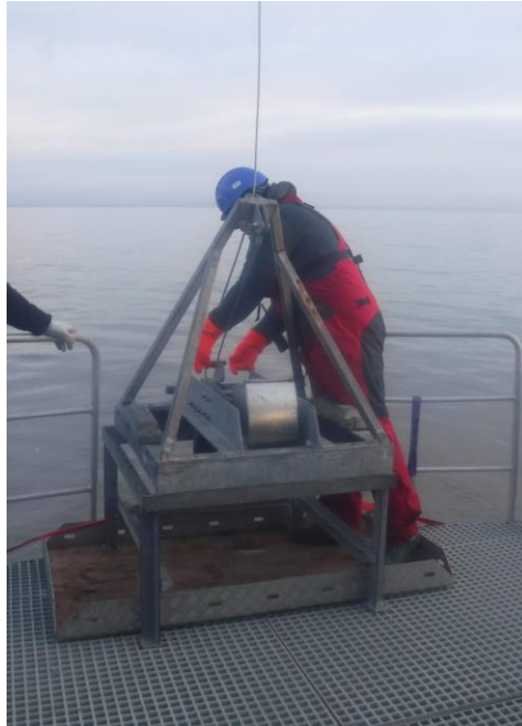
Mini Hamon grab being deployed from NWP 4 th / 5 th March 2020.
