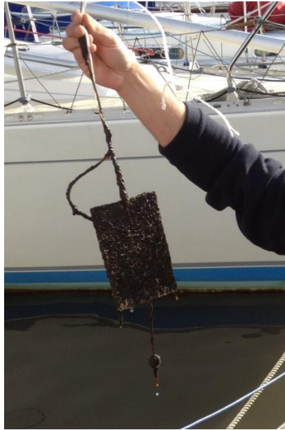
Figure 2: A settlement panel after 8 weeks of submersion, showing the arrangement of fishing weights (Photo: Hayden Hurst, CWT)
